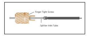
While holding the depth gauge, push the finger-tight screw up against the ferrule. Lock the screw into position by clamping the clear acrylic clamp onto the inlet tube.
