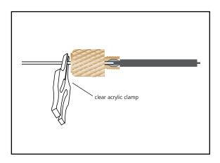
Remove the depth gauge. The screw and ferrule will now be in the correct position on the splitter inlet tube.
