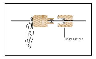
Tighten the nut and screw together and remove the clear acrylic clamp.
