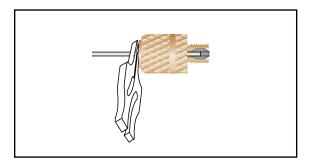
Slide the PEEK finger-tight nut onto the 1/16" tube that the splitter will be connected to. Insert the tube into the double–ended ferrule while holding the clear acrylic clamp (the clamp will stop the ferrule and screw from slipping out of position when the second piece of tubing is inserted into the ferrule).
