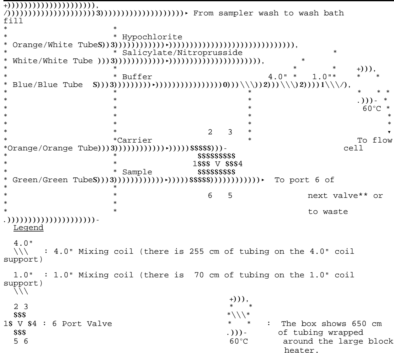
Figure 1. TKN Analytical Manifold (Lake and Rain Water)
