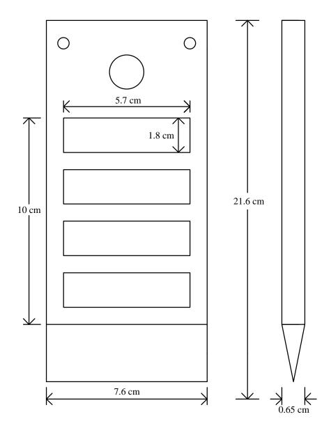
Figure 2. Top View of a Dry Deposition Plate
