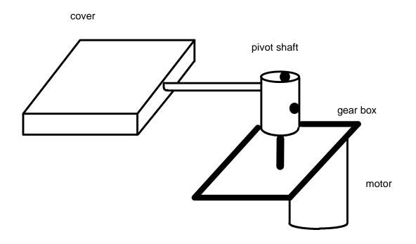
Figure 4. Top and Side View of Plate Cover
