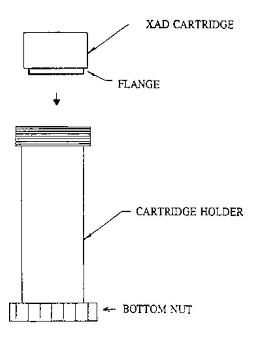
Figure 3. XAD-2 Cartridge and Cartridge Holder
