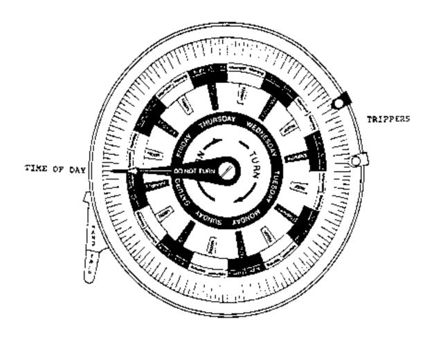
Figure 1. Mechanical Timer
