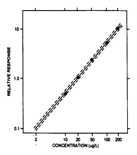
FIGURE 5 Relative Response Calibration Curve for Toluene. The Dotted Lines Enclose a  $\pm 10$  Percent Error Window.
