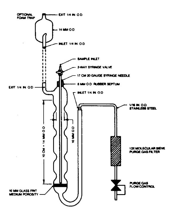
FIGURE 1 Purging Device.
