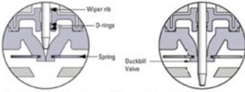
0-rings make sliding seal around needle
