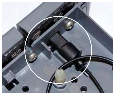
Figure 5 Column Outlet Fitting Installed in Column Cartridge
