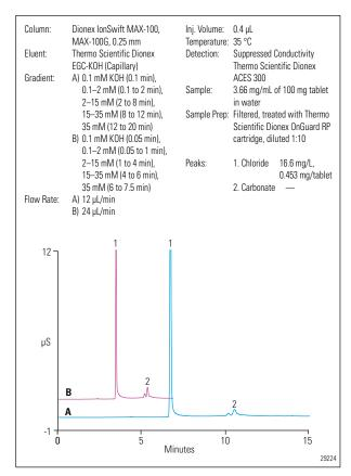
Figure 1. Capillary IC determination of the counterion in a drug used to treat type 2 diabetes.
