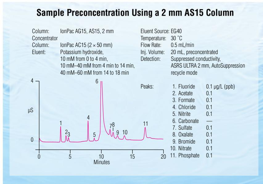
*IonPac® and IonSwift™ concentrator columns for anion, cation, and chelation ion chromatography are used to concentrate analytes, allowing determinations at µg/L (ppb) and sub-µg/L levels.*
