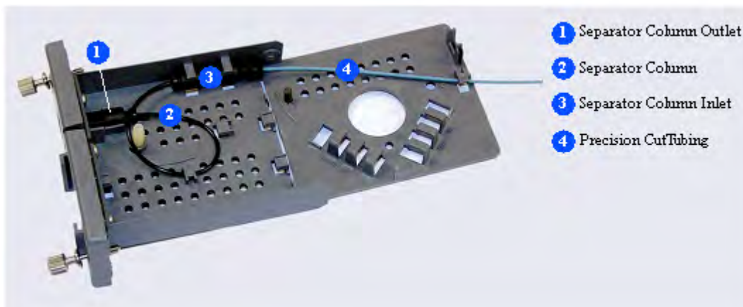
Figure 3 Separator Column Only Installed in Column Cartridge
