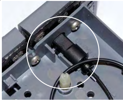
Figure 6 Column Outlet Fitting Installed in Column Cartridge
