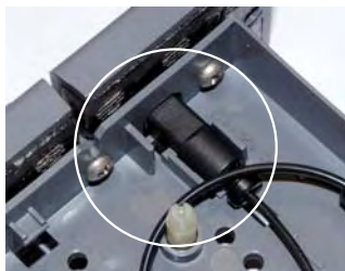
Figure 5 Column Outlet Fitting Installed in Column Cartridge
