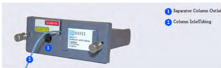
Figure 6 Column Cartridge Closed
