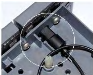
Figure 5 Column Outlet Fitting Installed in Column Cartridge
