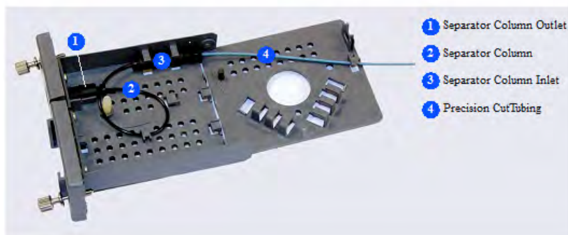
Figure 2 Separator Column Only Installed in Column Cartridge
