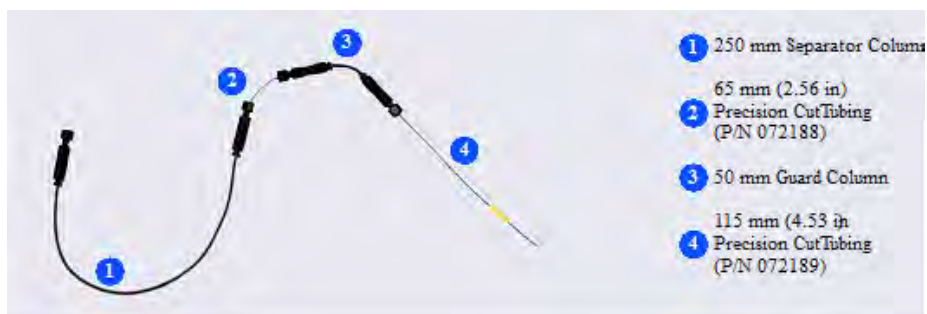
Figure 3 Tubing Connections for 250-mm Separator Column and 50-mm Guard Column
