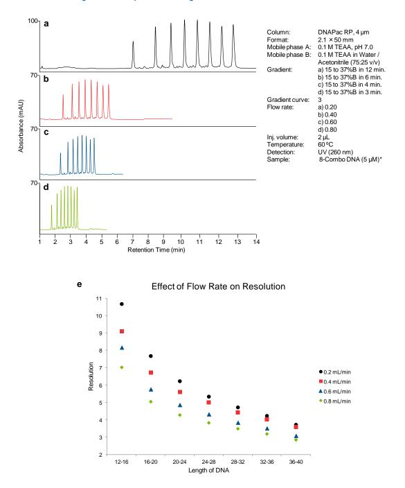
Figure 4. Separation of oligonucleotides at different flow rates
