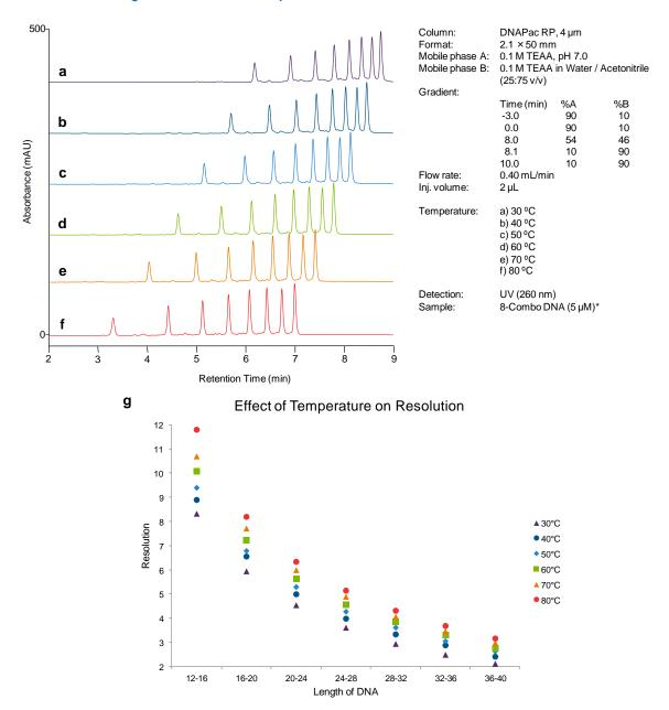
Figure 2. Effect of temperature on retention time and resolution
