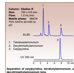
A mixture of cetylpyridine, tetrabutylammonium, and decyltrimethylammonium ions is shown on Obelisc R with mass spec compatible conditions. Cetylpyridine has UV absorbance, but ELSD is required to detect all three compounds.
